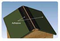
Apply roofing felt adhesive to both sides of the roof ridge to a distance of 150mm from the ridge on both sides.
