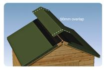
6 Cut a capping strip 300mm wide and with an overhang of 500mm to the back and front. Fix to the ridge pressing down onto the adhesive and dress down the roof 150mm each side.
