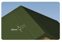
7 With the capping strip in position nail the lower edges at 50mm intervals. Carefully fold over the ends and secure with nails.
