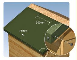
Fix in position by nailing the top edge of the felt with 13mm galvanised clout nails at 500mm centres. Slowly and carefully fold overhangs over the edges of the roof and nail at 75mm intervals. Fold and nail corners to make a neat appearance.
